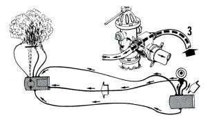
Line is connected from pump discharge valve to bring intial supply line up to pump pressure.
