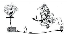
First engine drops preconnected valve at the hydrant and stretches line to the fire. Valve is connected to the hydrant, smaller chamber is positioned up or down depending on location of fire and hydrant is opened.
