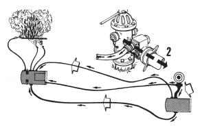
Second engine lays two lines from fire to hydrant, connects sleeve to valve to supply those lines through the pump.
